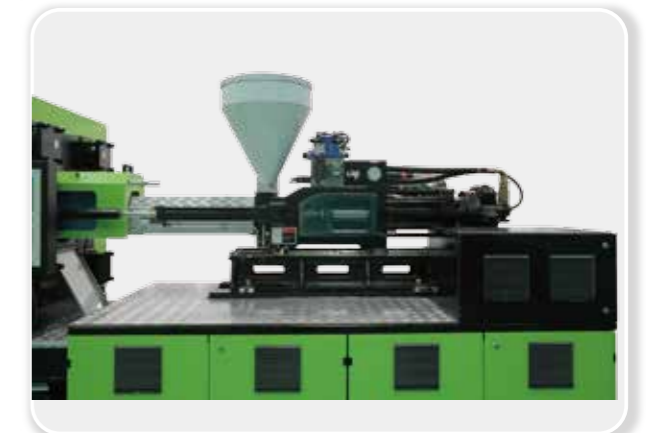
Single-cylinder injection system with high precision
